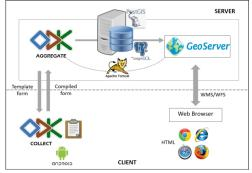
Figure 1: System architecture
