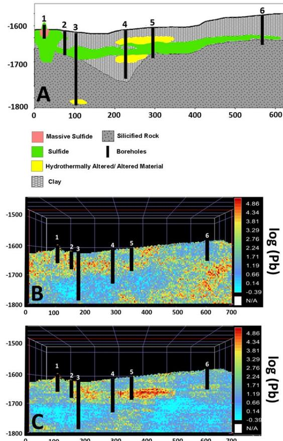
Fig. 2: Cross-sections along E-W in which (A) illustrates the conceptual model of study area, and (B) and (C) depict spatial distributions of  $\log(\text{Pb})$  using Sequential Gaussian Simulation (SGS) and Turning Bands Simulations (TBSIM), respectively.
