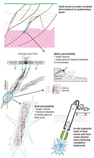
Figure 1. Conceptual diagram of permeability and porosity testing scales on drill core and in-situ in fault zones under sedimentary basins that may host geothermal resources. Modified after Scibek (2019, 2020).
