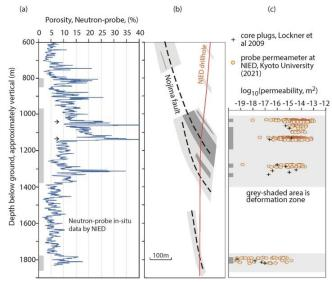
Figure 2. Example of fault zone properties at NIED drill hole, Hirabayashi drill site, Awaji Island. (a) Neutron-probe in-situ porosity, NIED data, and (b) drill core rock matrix permeability tested by Kyoto University.
